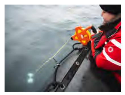
This project supports the Secchi Disk Foundation and is named after the white disk that measures the clarity of the seawater. A Secchi Disk will be used to record the Secchi Depth and will be lowered vertically into the seawater from the Zodiac.
